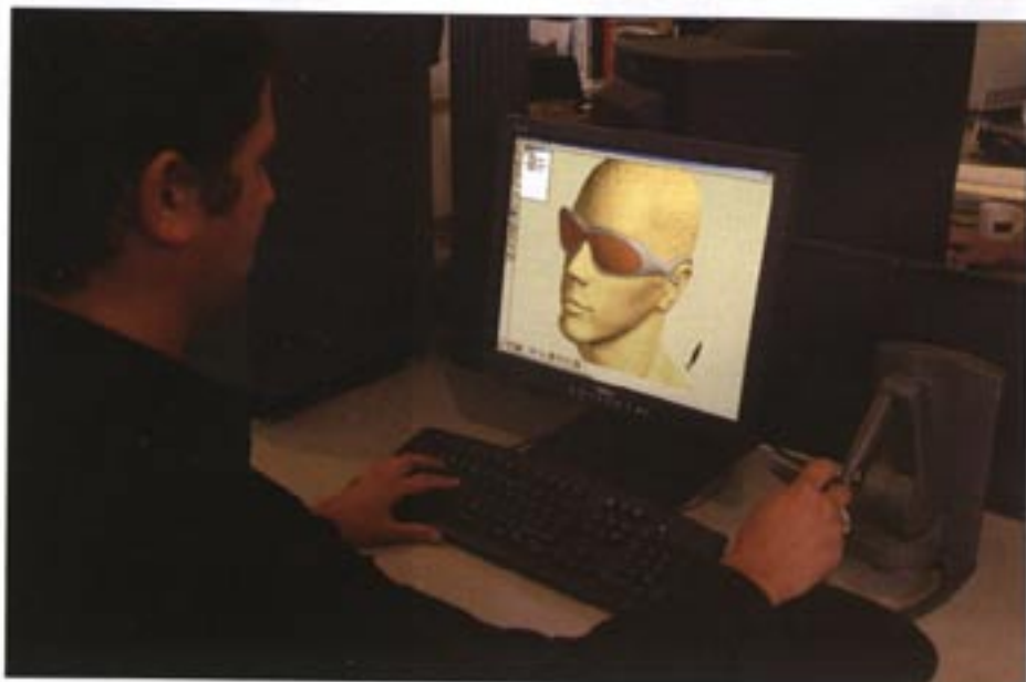
PDD's design studio uses SensAble FreeForm, a touch-enabled system that gives designers a quick, easy way to develop realistic conceptual designs in 3D
